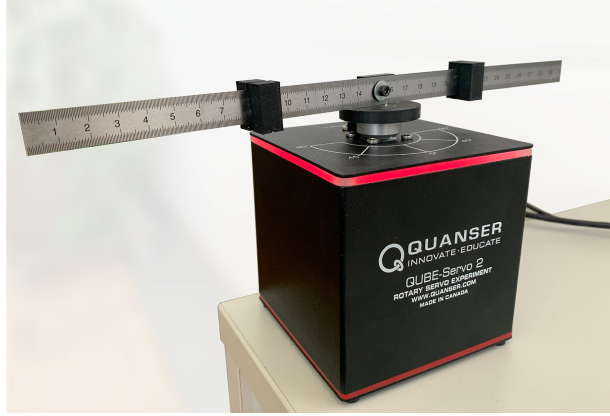
Figure 1: System under consideration: DC motor with a rotary flexible link
